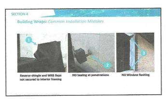
SECTION 4 **Building Wraps: Inspection**  Visually inspect if WB system was correctly installed per manufacturer's Requires periodic field observation reports for quality assurance and special warranty documentation Visually inspect building wrap air barrier for proper > Continuity, > Overlap, COFF > Flashing and > Fastening prior to covering it with cladding
